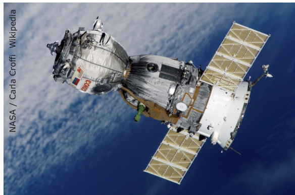
TMA Spacecraft capable of ferrying three cosmonauts to and from the International Space Station.
